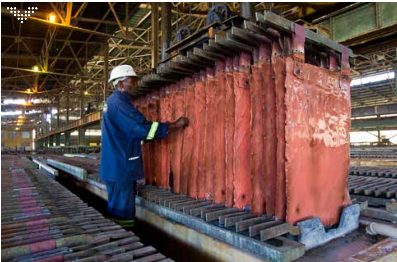
Production of copper plates by electrolysis
